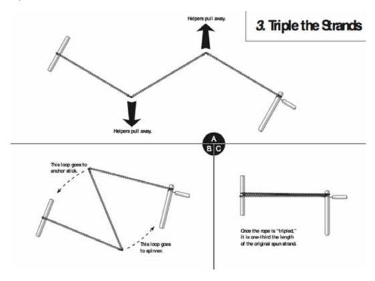
Next the newly tripled rope must be wrapped or twisted as before, BUT now it will be wound the opposite direction to make the rope fibers grab onto each other so that they won't unwind once tension is released. Once the tripled rope is wound tightly the opposite direction of the original twist it should be pulled back and forth in a quick motion to set the rope fibers.
