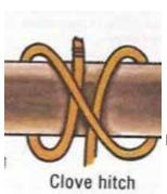
Uses: Ties a rope to a tree or pole
