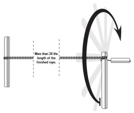
Lastly the rope can be relaxed and removed from the dowels it is attached to. The ends can be taped, whipped, or back spliced to prevent them from fraying.
