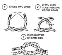
Uses: Joining two ropes together "Right over left and under, left over right and under"
